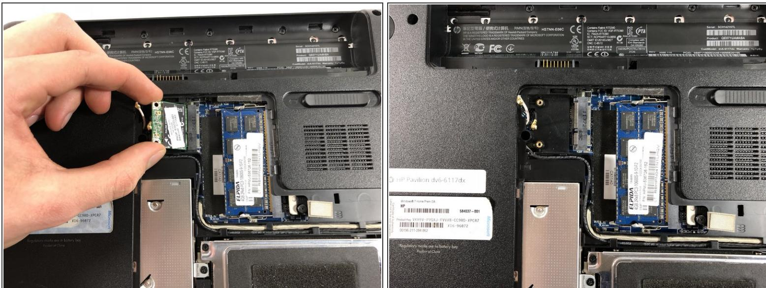
! Always handle the WiFi Adapter by the edges to avoid damaging the part.
