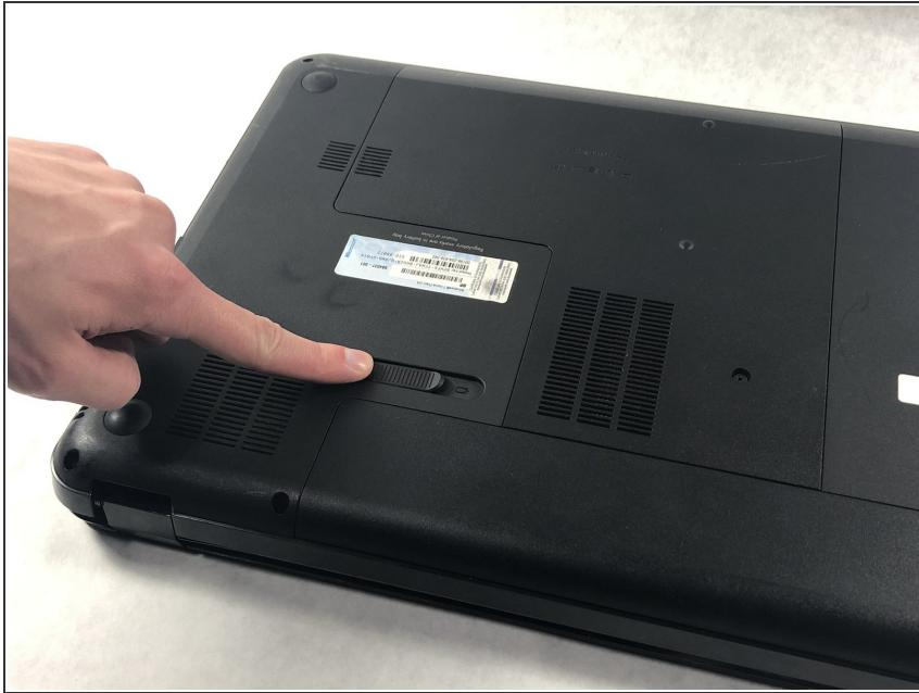
**⚠** Shut off your device and disconnect the power cord. Disconnect any external devices connected to the device.
