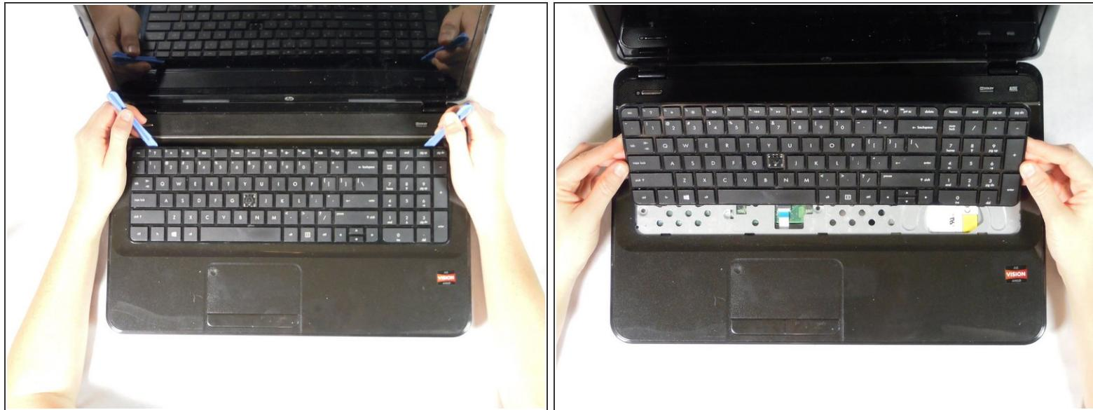
**⚠** A ribbon cable is attached to the back of the keyboard. Avoid lifting or moving the keyboard more than a couple inches before you disconnect the ribbon cable or you may damage it.
