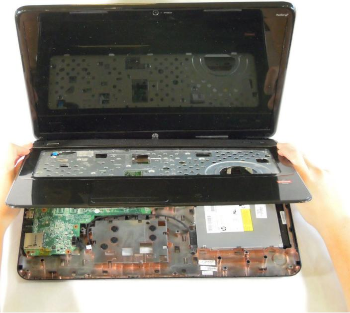
**⚠** Lifting the top panel too quickly or forcefully may damage the speaker cable, which is still attached underneath.
