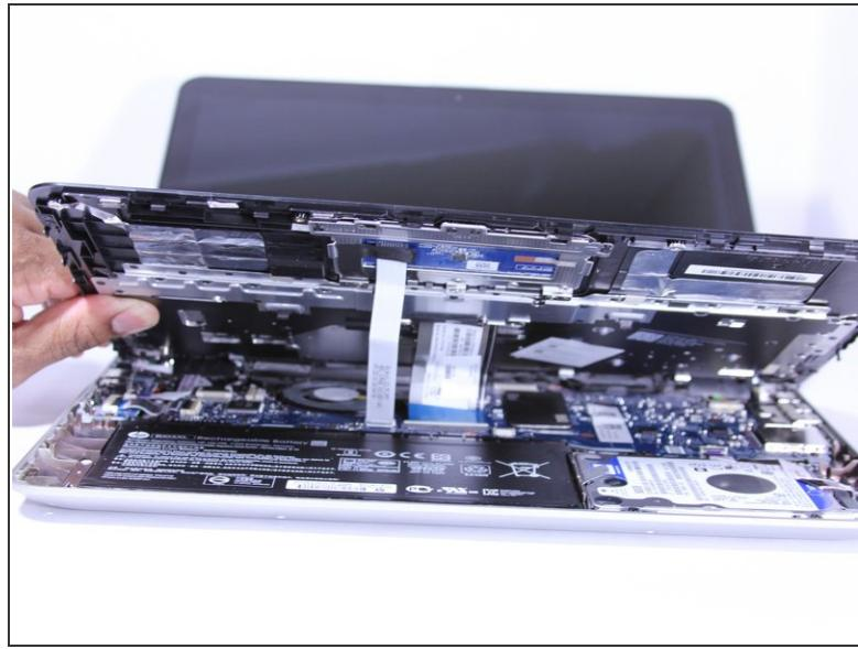
**⚠** The keyboard is attached internally by clips. Use a small amount of force when removing the keyboard.
