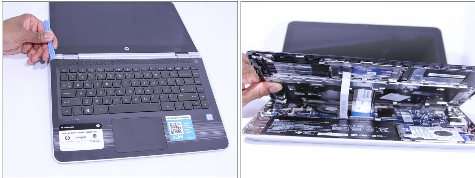
**⚠** The keyboard is attached internally by clips. Use a small amount of force when removing the keyboard.
