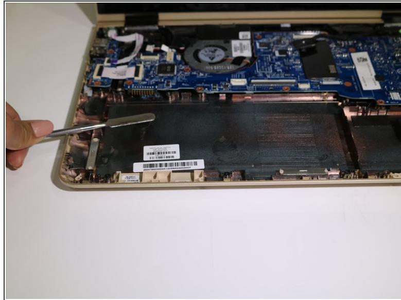
**⚠** Carefully pop out the battery using the silver Metal Spudger to disconnect it from the motherboard.
