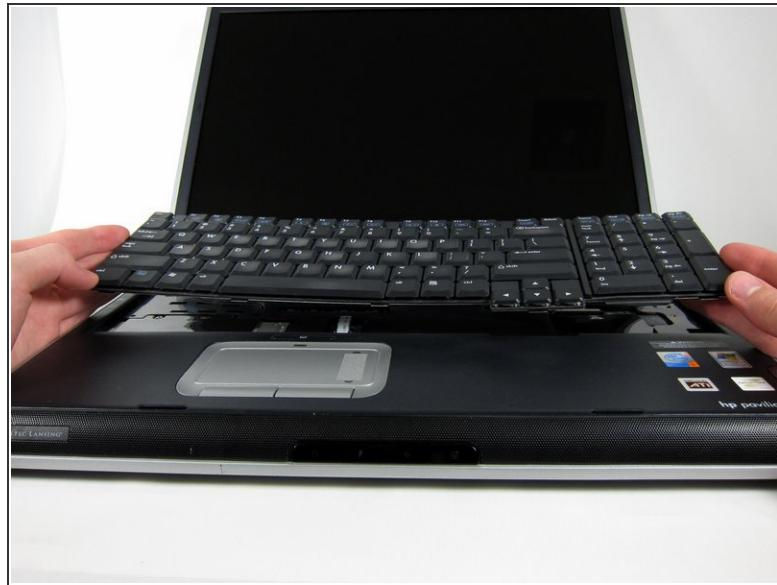
⚠ Lift the keyboard carefully because it is attached to the motherboard by a ribbon cable.
