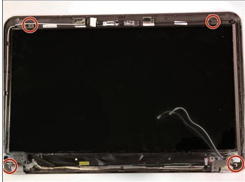
⚠ Gently flex the inside edge of the top, sides and bottom of the display until the bezel disengages.
