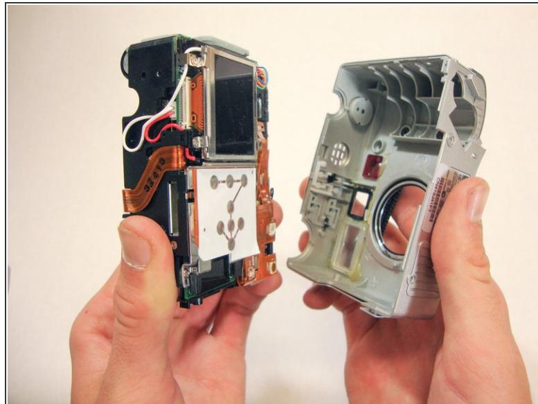
**⚠** While pulling the camera out of the case, note the small soft plastic cover on the side of the camera. This cover will detach from the rest of the device.
