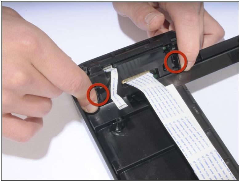
*(i)* The LCD screen is attached to the piece of the hood with the glass shield.
