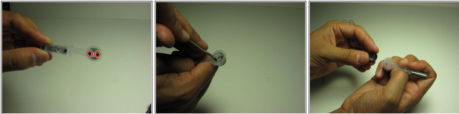
ⓘ The plastic holder secures the power button by two slots.
