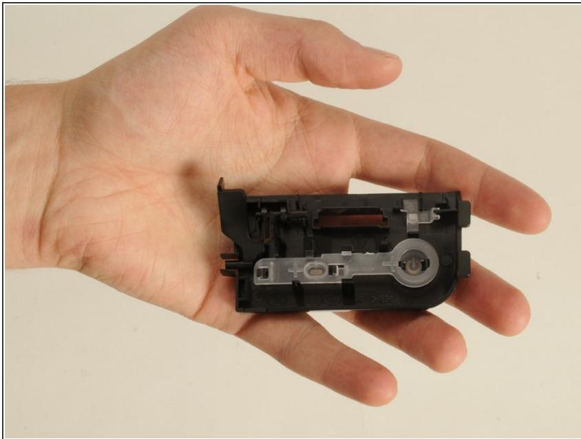
**i** A picture of the removed power button is provided to show the location of the clip that needs to be pressed.
