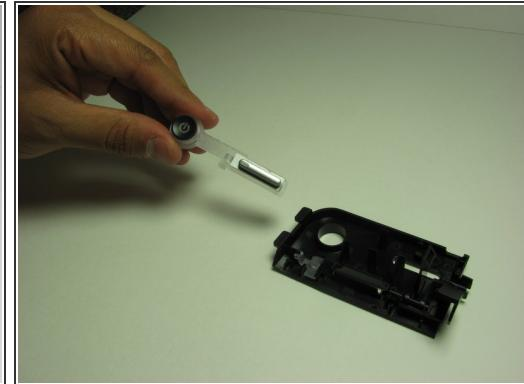
**i** The power button face has a plastic holder that attaches the power button and the wireless button to the face plate using two slots.
