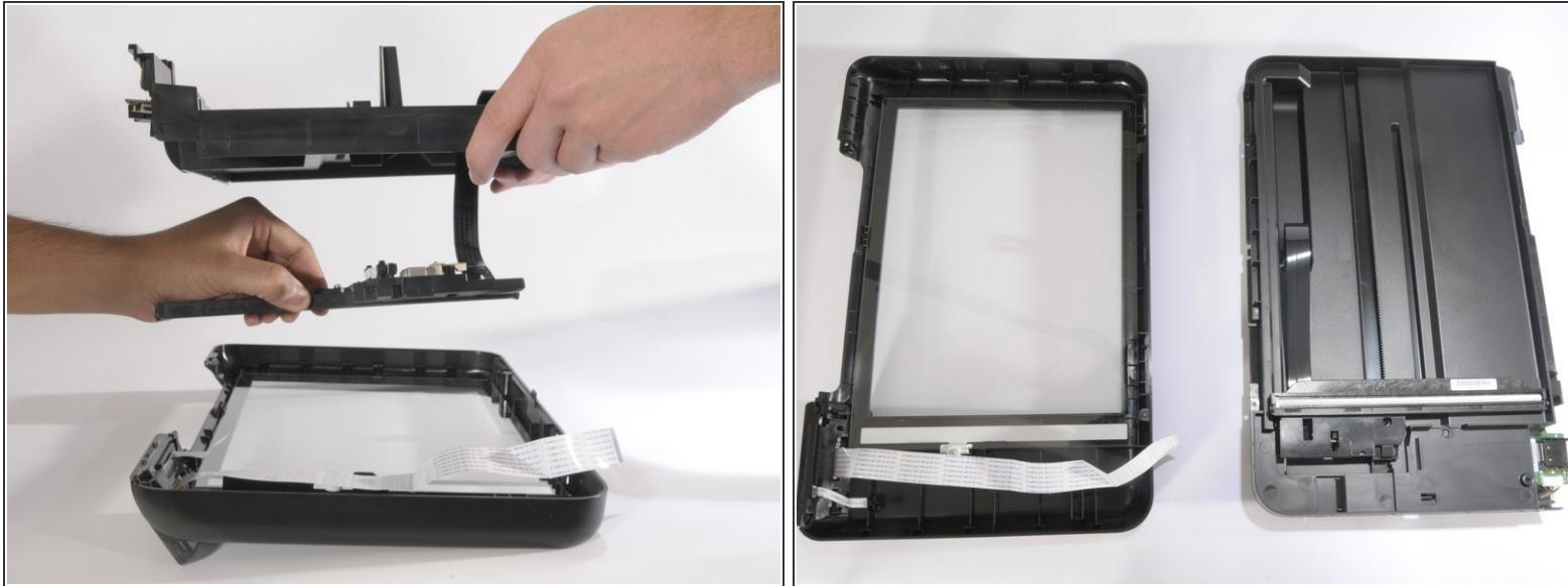
**⚠** Carefully separate the two hood pieces connected by the black ribbon.
