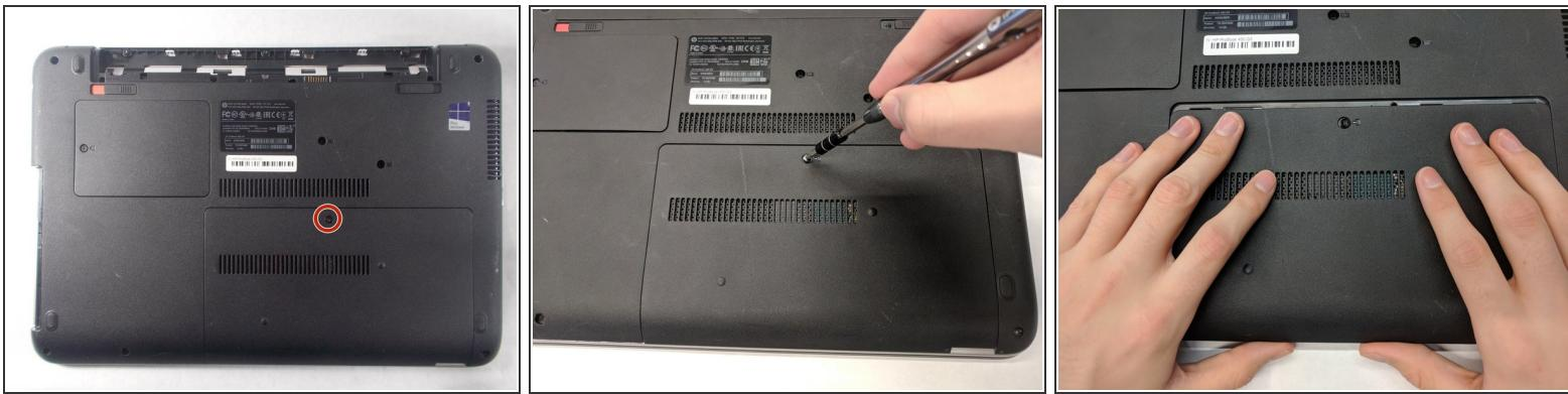
*(i)* The screw is not supposed to come out. It is there to hold the case down.
