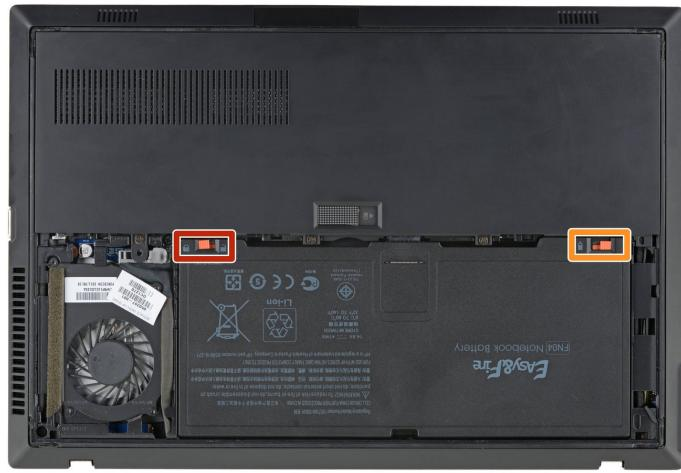
ⓘ Two switches lock the battery in place. To remove the battery you will need to slide both switches toward the center of the battery.
