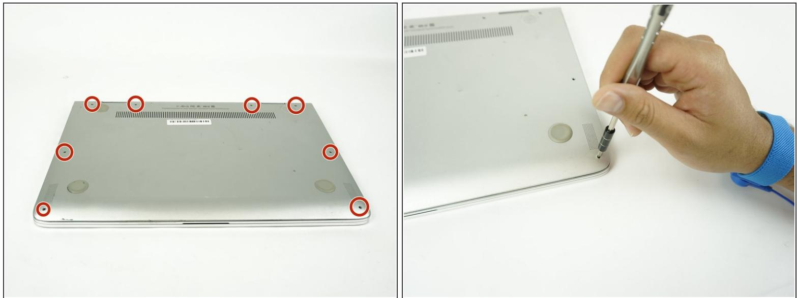
**⚠** Static buildup and discharge can damage your computer's components. Use the Ant-Static Wrist strap to help prevent this.
