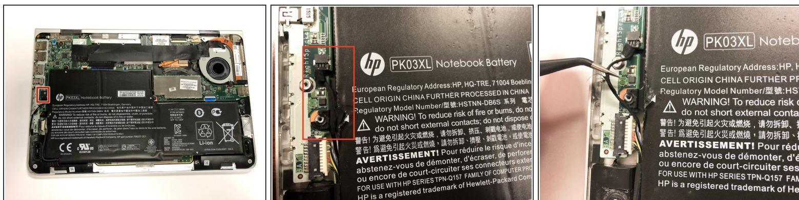
**⚠** Do not disconnect the cable connector shown in the red box.
