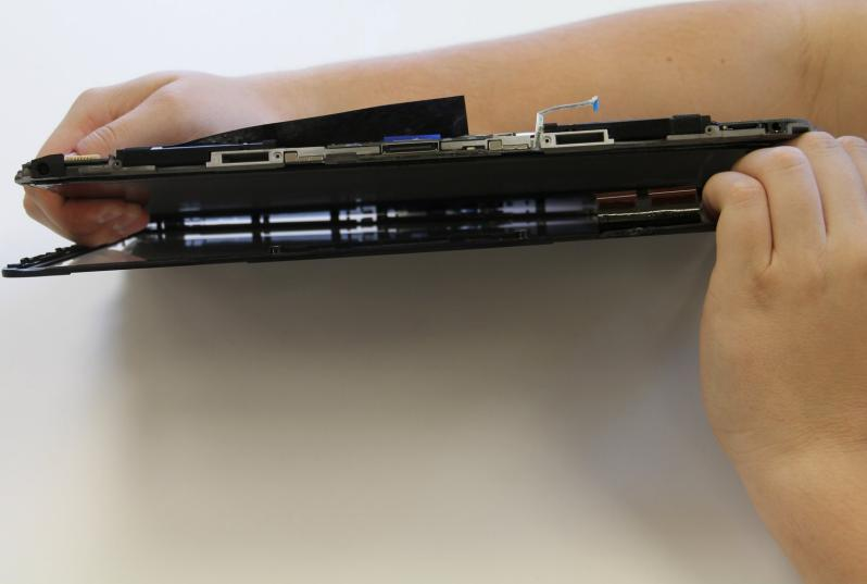
ⓘ Glue is holding the device together along the edges. The glue is can be very strong. A heat gun may be required to loosen the glue for removal of the digitizer to prevent damage to the screen.
