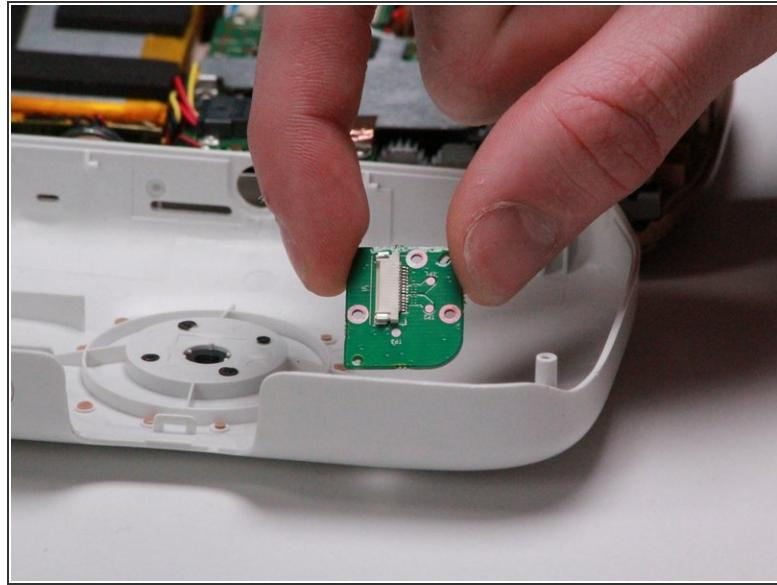
⚠ Carefully remove ribbon from the flash circuit board.
