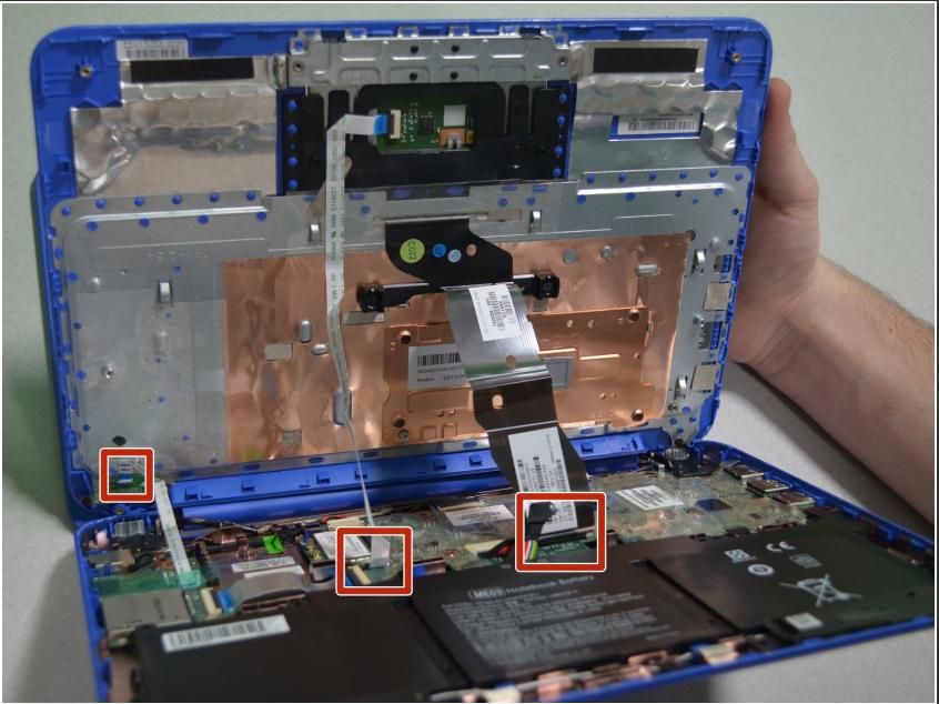
⚠ Slowly lift the keyboard as there are multiple ribbon cables that could easily be damaged if lifted with force.
