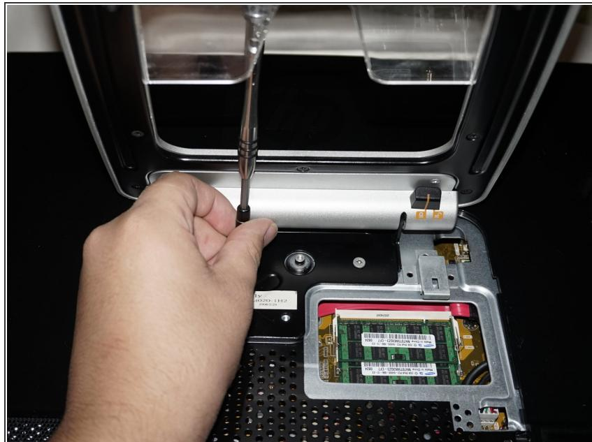
*(i)* The top hinge screws can be difficult to get to. If you are using the classic iFixit screwdriver handle, the best workaround to this problem is to put the extension on and twist this part to remove the top screws. This is not required for the bottom screws.
