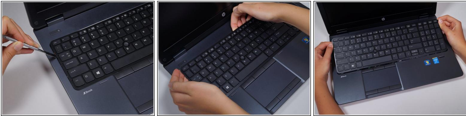
**⚠** Do not try to pry the keyboard from the bottom. The keyboard is attached by clips on the left, top, and right side. Metal inserts on the bottom side lock the keyboard in place until they are slid up and out.
