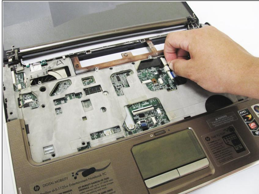
**!** The display should now be loose, but make sure to remove all ribbon connectors before attempting to take off the display.
