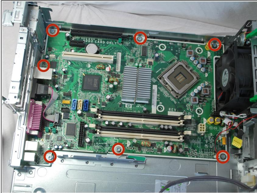
**⚠** Make sure everything is removed and/or disconnected, including the heat sink, the CPU, and all connecting cables.
