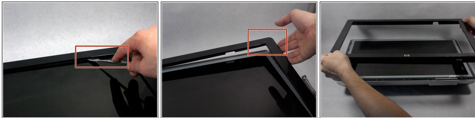
**⚠** Do not put the metal spudger between the metal and the glass. It needs to go under the bezel and above the metal.
