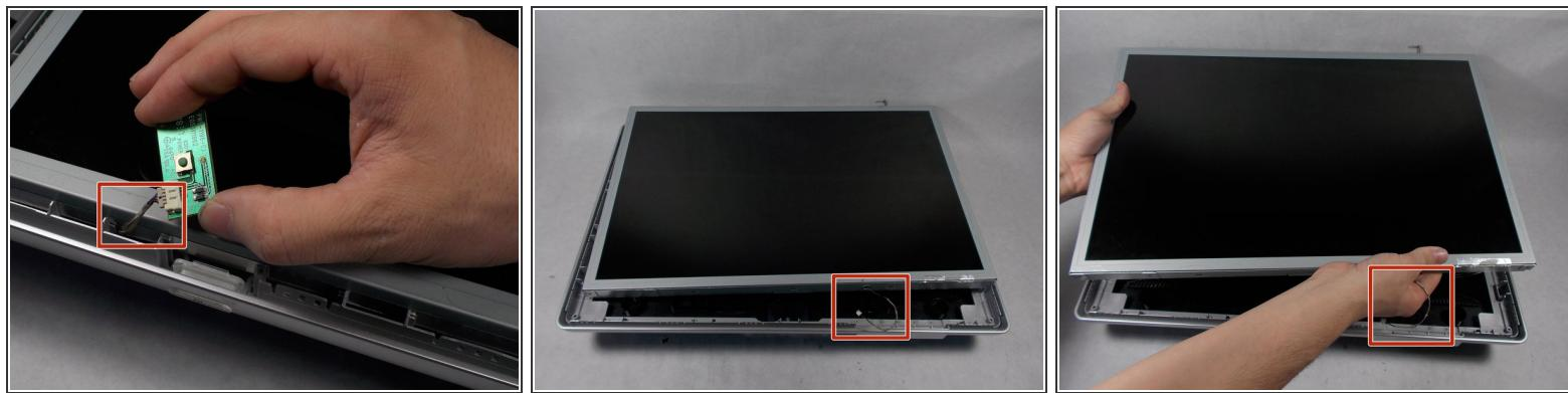
**⚠** Be careful of the wires attaching the power button and the control buttons. Show extreme caution to ensure the button is not damaged.
