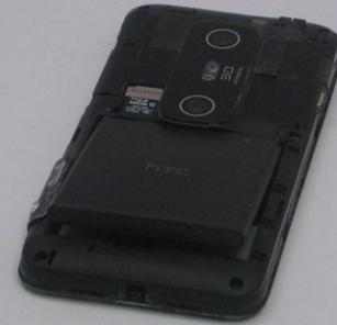
*(i)* When insert the new battery, be sure to align the golden contacts on the top part of the battery compartment with the replacement battery.
