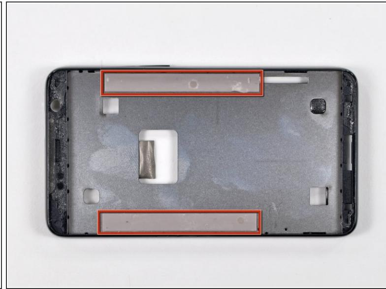
ⓘ In the following steps, you will use a heat gun to soften the adhesive securing the underside of the LCD panel to the inner case. The area the adhesive is applied to is shown in red in the second picture (with the LCD removed).
