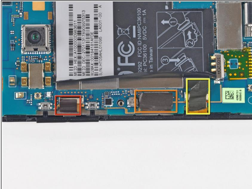
*i* Fold the device information sticker up against the top of the motherboard to keep it out of the way while you work.
