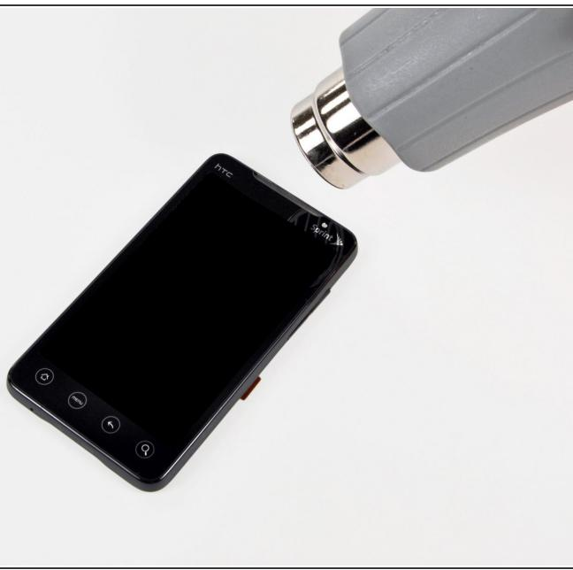
**i** In the following steps, you will use a heat gun to soften the adhesive securing the outer black border around the underside of the front glass panel to the inner case.
