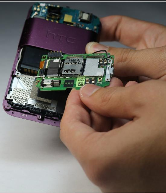
**⚠** Carefully remove the motherboard from the base of the phone.
