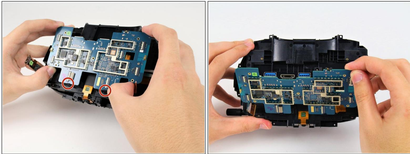
! The bottom of the motherboard is secured by two hooks, indicated in the first photo. Do not pull the motherboard directly outwards, as doing so can cause damage.
