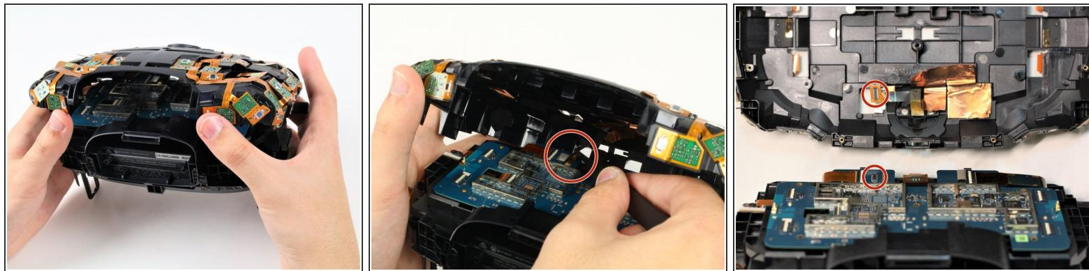
**⚠** Be careful not to lift the sensor array too far from the rest of the device because the camera ribbon cable may tear.
