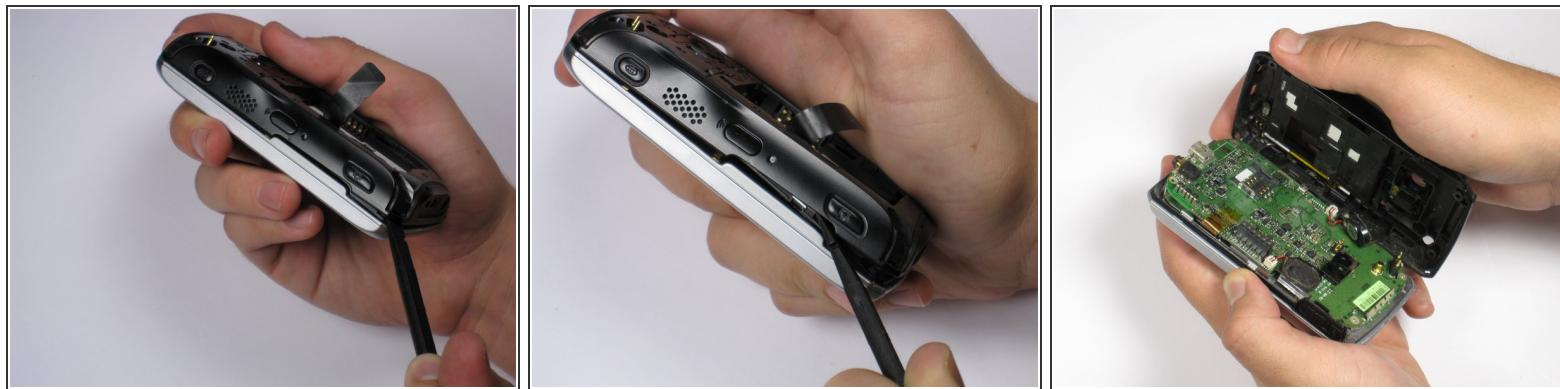
**⚠** Be Careful! Do not insert the spudger in between the keyboard and screen. This could break the keyboard off the phone.
