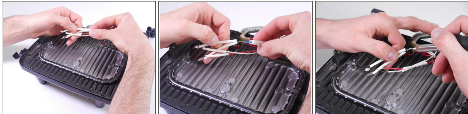
**⚠** Very gently, slide the white wiring covers down to expose the wiring connectors
