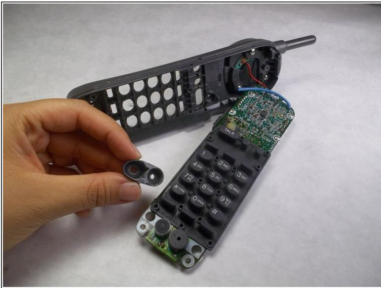
*(i)* After disassembling the handset, you will see the inner components of the handset.
