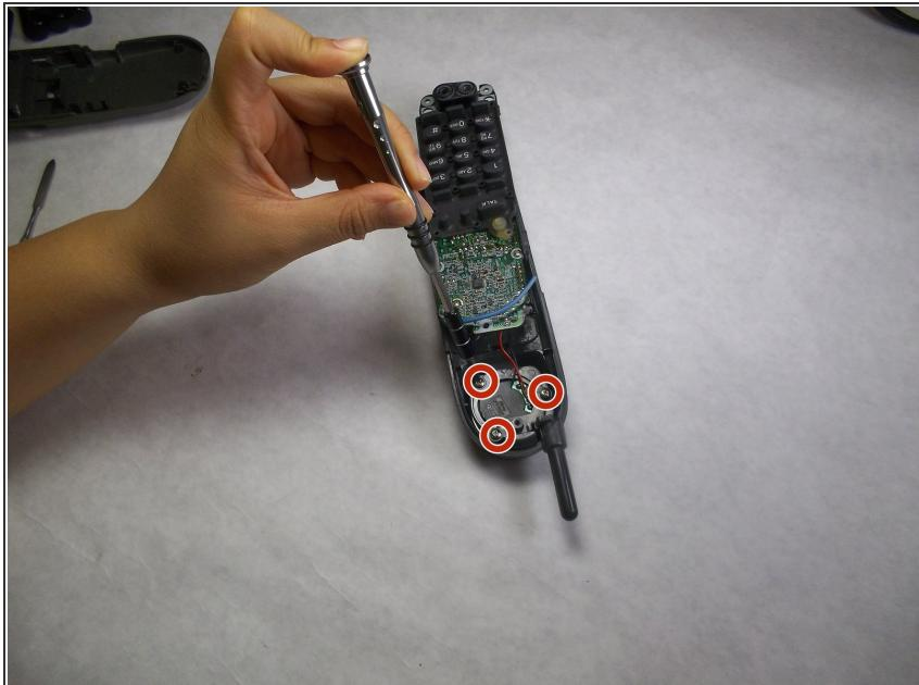
*i* After disassembling the handset, you will see a circular component at the top section of the handset. This is your speaker.
