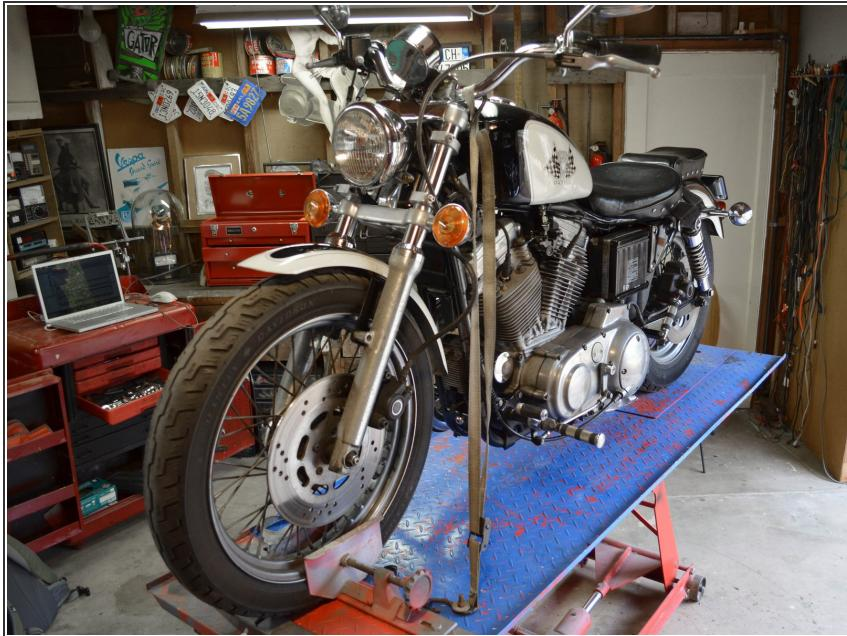
When working with the brake lines, we strongly recommend using a bike stand or similar apparatus to stand the bike upright and lock the front tire in place.
