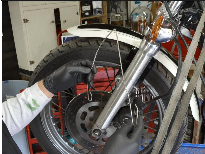
*i* Allowing the brake assembly to dangle from the brake lines can cause damage to the line.
