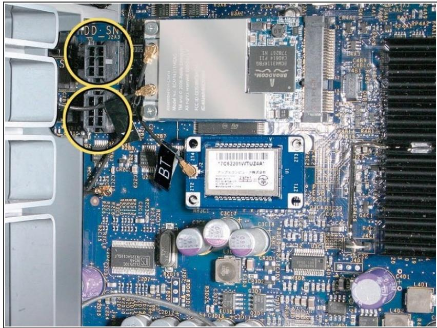
**Replacement Note for Card Using One Booster Cable:** Be sure to connect the card's booster cable to the correct auxillary power connector on the logic board. Connect the booster cable for a card in PCI slot 1 to the lower connector. Connect the booster cable for a card in PCI slot 2 to the upper connector.
