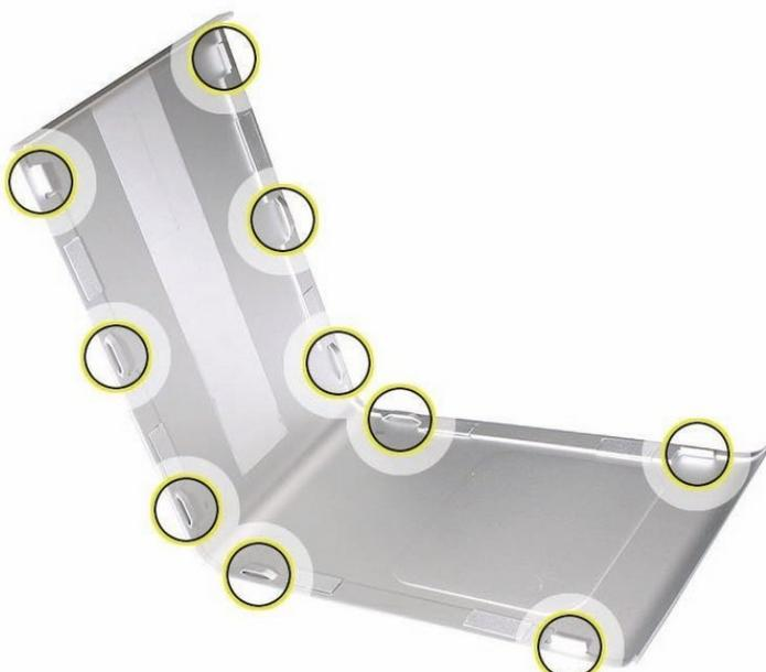
**Replacement Note:** When reinstalling the processor heatsink cover, make sure the tabs on the underside of the cover align with the slots directly below them. (The slots are on the front fan and memory cage on either side of the heatsink cover.)
