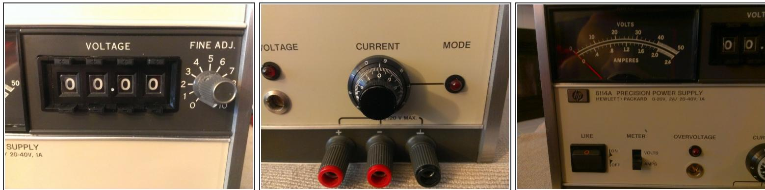
**⚠ Caution:** The power supply contains very large capacitors that can remain energized for extended periods of time. Touching the capacitor wires may cause serious injury. Use a [capacitor discharge probe](#) to safely rid the capacitors of dangerous charges.
