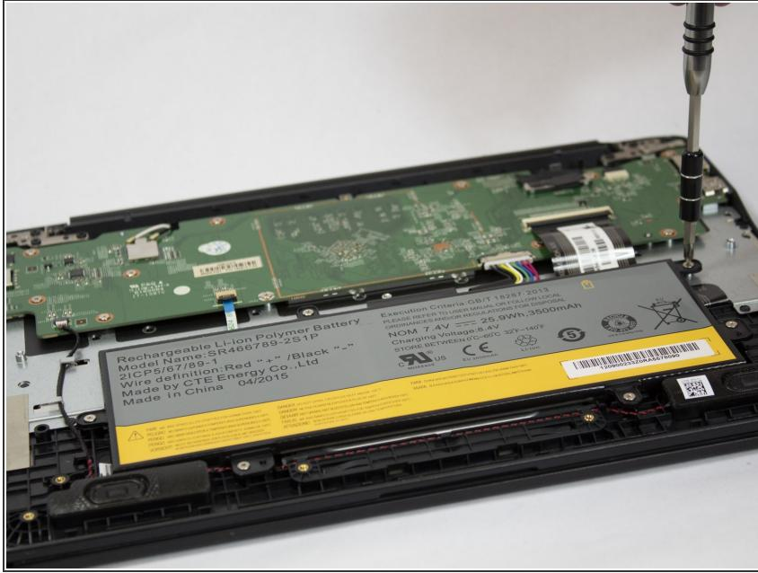
! Be careful not to puncture the battery with the screwdriver or any sharp instrument.
