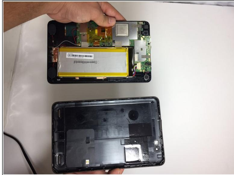
*(i)* Turn tablet off before disassembling it.
