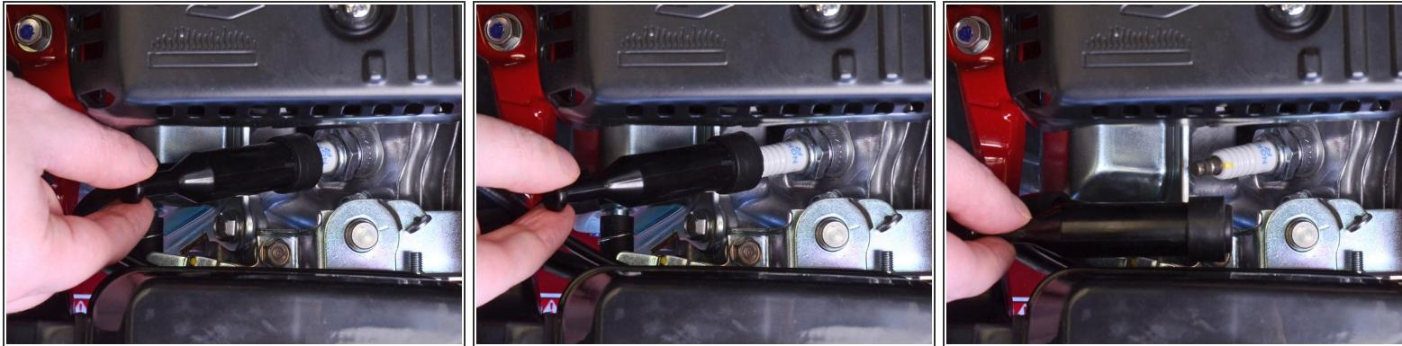
! Before you begin, it's important that you completely cut power to the tiller by disconnecting the spark plug. This will prevent the engine from accidentally starting up while you're working on the tiller.
