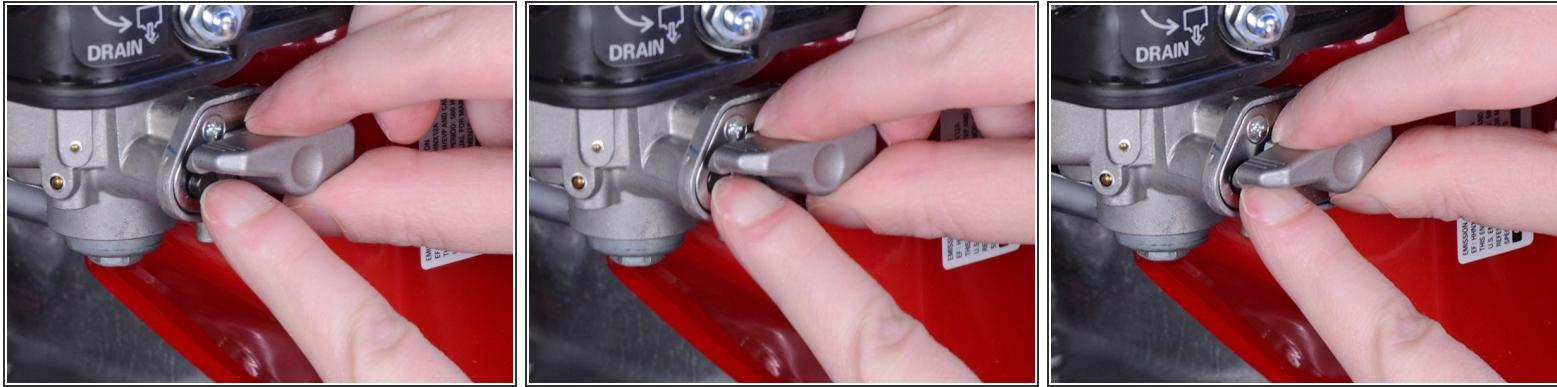
ⓘ The next two steps demonstrate how to empty gasoline out of the carburetor before removal.
