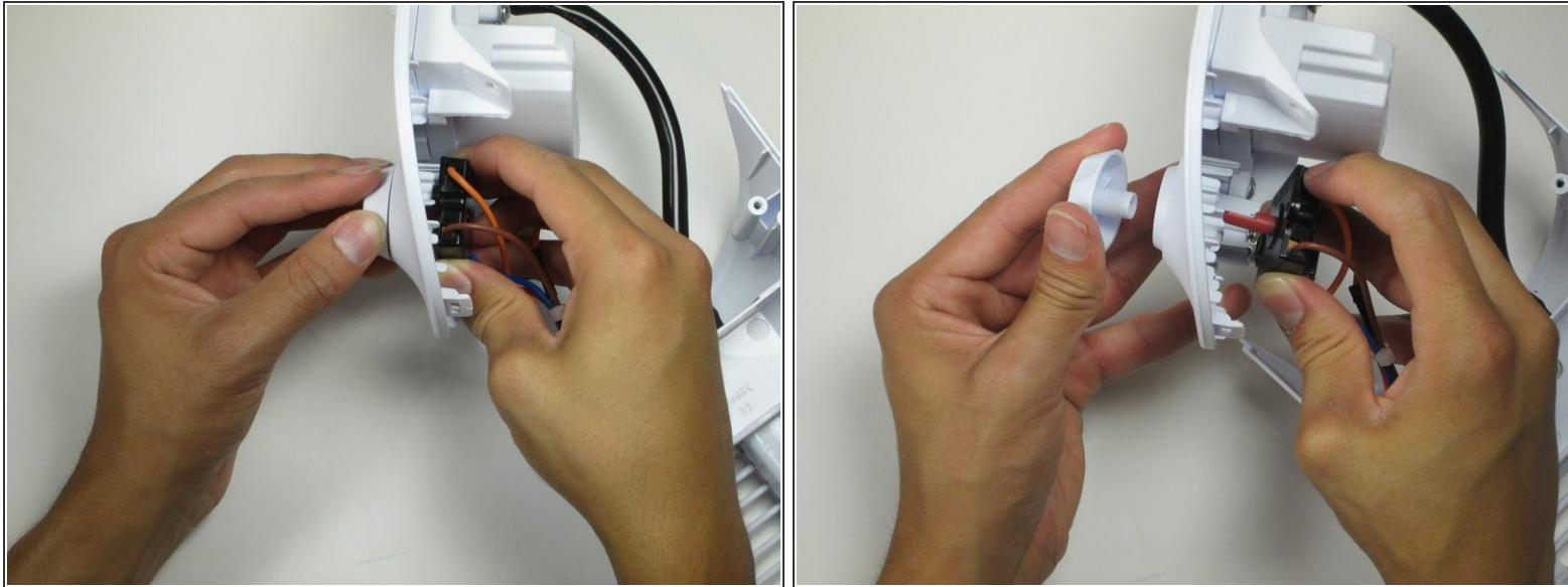
**⚠** Be careful not to separate the wires from the black dial box during separation, or you will have to re-solder them.
