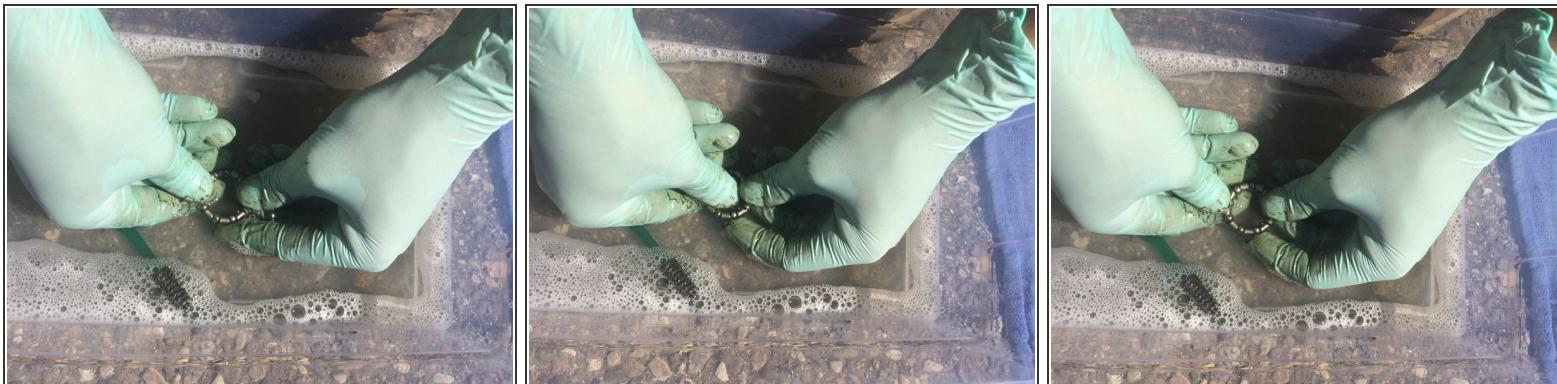
● When cleaning the bearings, spin the balls to help remove grit from inside.
