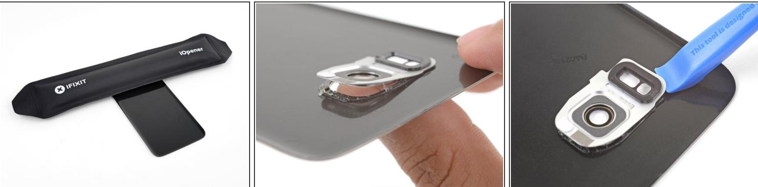
ⓘ The following four steps show how to remove and transfer the rear bezel. The bezel supports the rear cameras, flash, and the fingerprint sensor (on some models).
