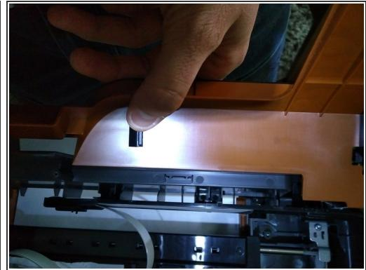
! Next, remove the orange cover. Use caution as the display unit is still attached to the cover. If you pull the cover off too quickly, you could tear the flat cable.
