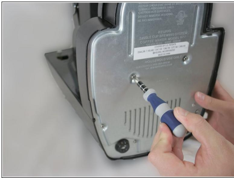
**⚠** Before beginning the repair, turn off the brewer and disconnect it from any power source.
