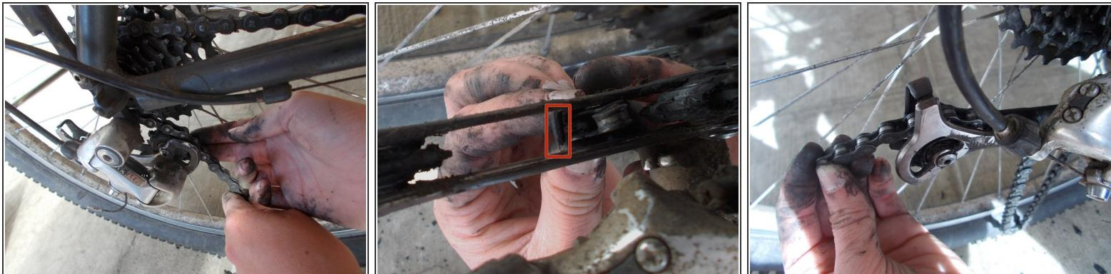
*(i)* If the chain fell off the rear derailleur, it needs to be re-fed through the proper pulleys.
