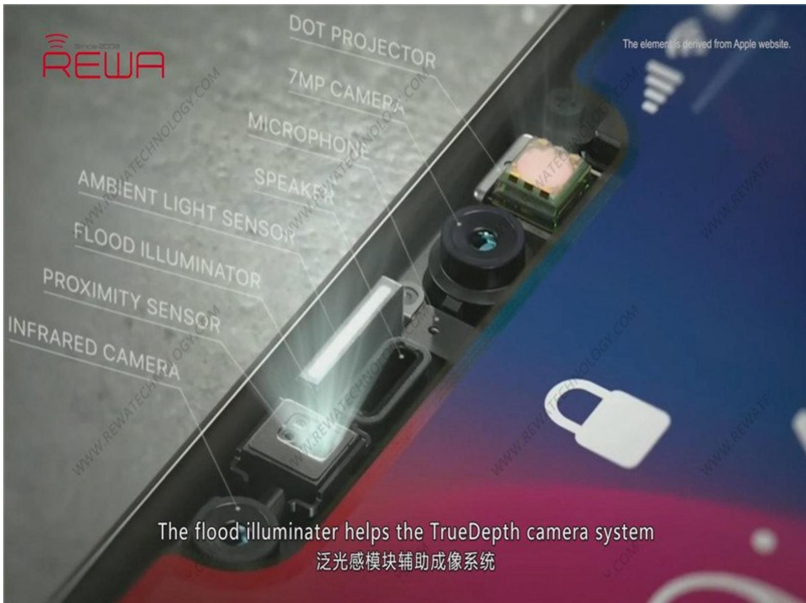
The flood illuminator helps the TrueDepth camera system
