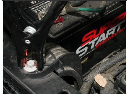
**⚠** Be careful with the booster cable clamp in order to avoid damaging your vehicle and getting electrocuted and NEVER allow the red and black cable clamps to touch each other.
